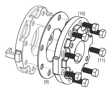
Step 2: Fasten the assembled Flange Adapter to the pump discharge, inserting the *3" Gasket [8]*. Three of the socket head cap screws that fasten the volute to the pump motor must be removed. <u>Do not</u> remove the screw opposite of the pump discharge.
