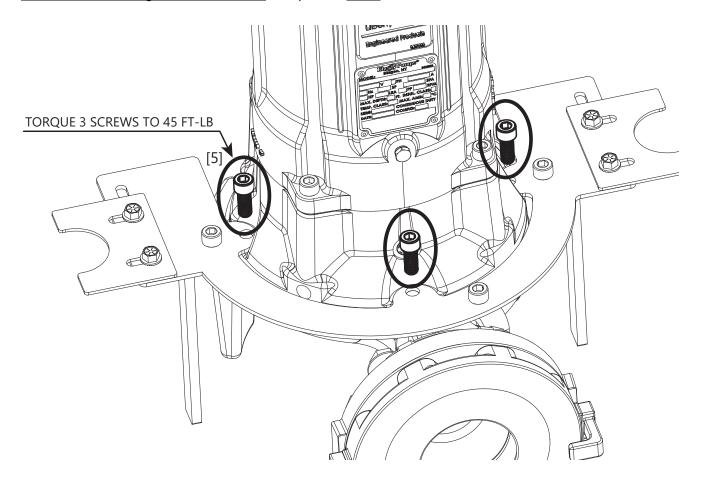
**Step 5**: Guide Plate Adjustment: The guide plates are adjustable to account for system installation variations and wear or corrosion. Guide Plates can be adjusted fore and aft and also inboard or outboard. Start with the edge of the Guide Plate lined up with the discharge facing edge of the Adapter Bracket. Both Guide Plates should also be moved out as far as possible.
