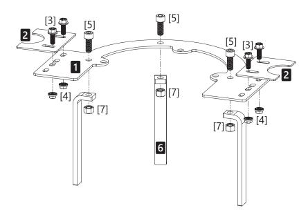
Step 4: Install the Guide Bracket Assembly on the pump. In order to do this, the pump should be lifted about 2" off the ground, or tipped on its back (discharge facing up in the air). Fasten the Guide Bracket Assembly to the pump using the provided 1/2-13 Socket Head Cap Screws [5].
